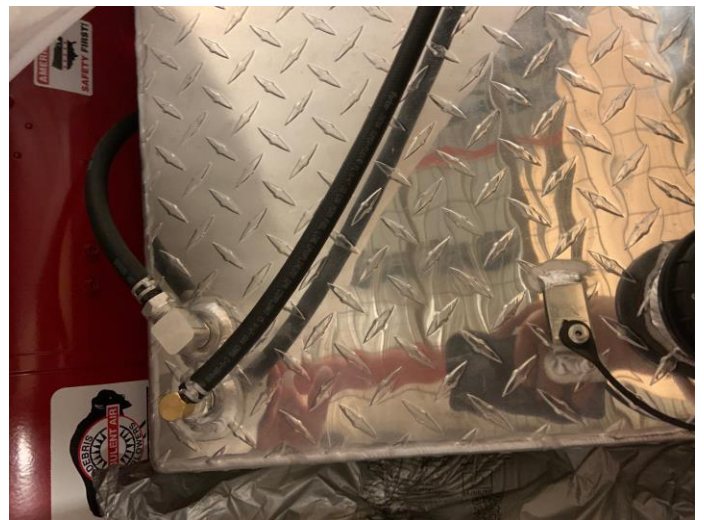
Step # 4: Install fuel line and clamp onto vent elbow fitting.
