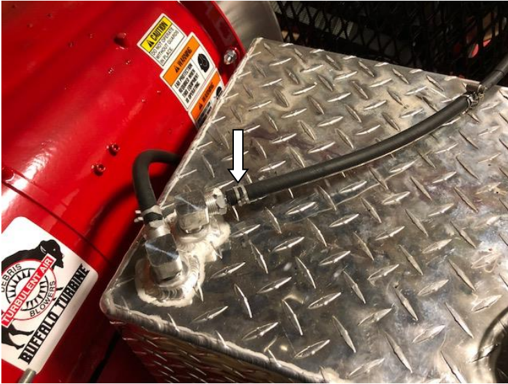
Step #3: Install Aluminum fitting into fuel tank first. Then install brass check valve.
