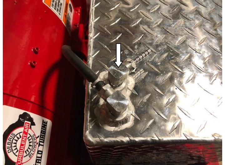
Step #2: Remove vent fitting from fuel tank
