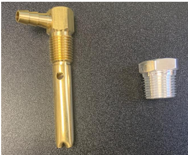
Step #3: Install Aluminum fitting into fuel tank first. Then install brass check valve.
