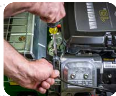
FIGURE 20A: THROTTLE ADJUSTMENT, COARSE (PHILLIPS SCREW) - Adjusting the position of the throttle cable outer sleeve
