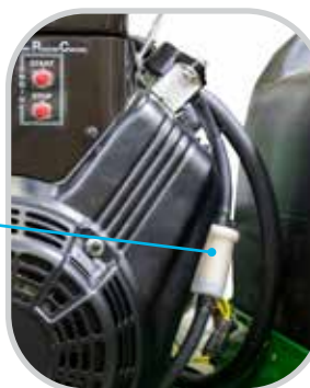
4 Fuel Filter* (spare part, not of Engine Assembly) Fuel Filter is on the side of engine.
