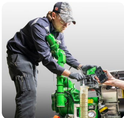
FIGURE 32: MEASURING THE ACTUAL FLOW
