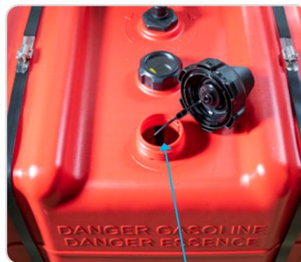
FIGURE 16: 1800E GASOLINE TANK, LARGE KNOB IS GAS FILL
