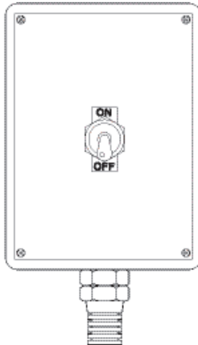
Figure 4 - Remote Control Station
