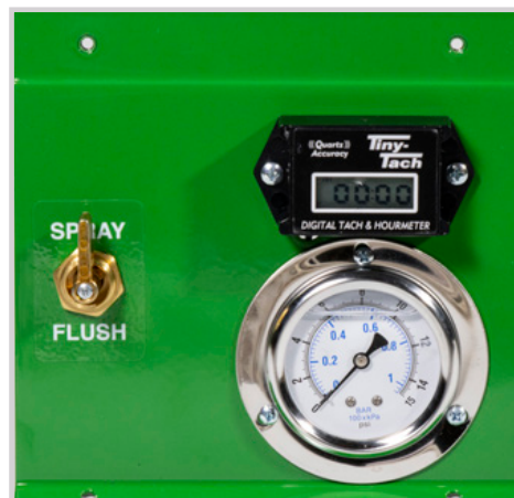
FIGURE 26: PRESSURE GAUGE SPRAY/FLUSH VALVE SWITCH
