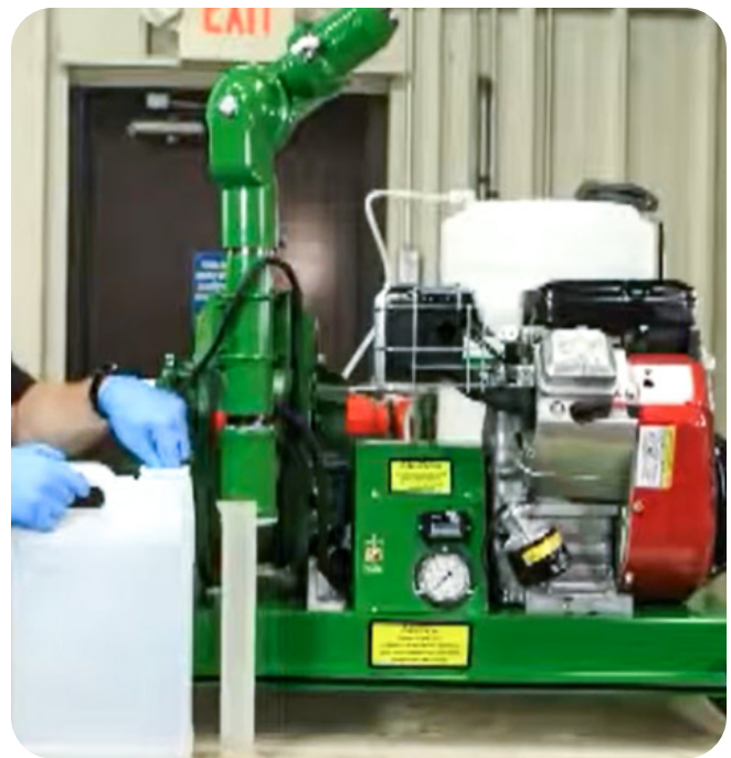
FIGURE 31: DISCHARGING AIR BUBBLES
