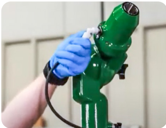
FIGURE 30: DISCONNECTING INSECTICIDE LINE
