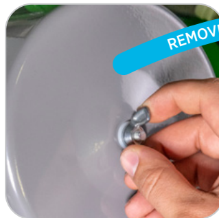
Remove wing nut from filter cover
