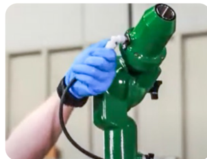
FIGURE 33: RECONNECTING INSECTICIDE LINE
